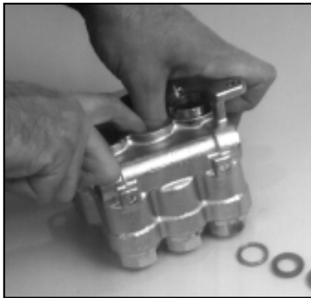
Installation of Male Adapter
