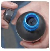
Remove black protective cap to expose male garden hose thread and internal checkvalve.
