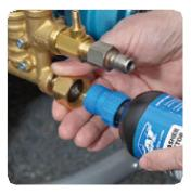
Screw bottle into garden hose fitting on inlet of pump.
