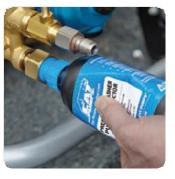
Squeeze bottle to inject pump protector fluid into pump.
