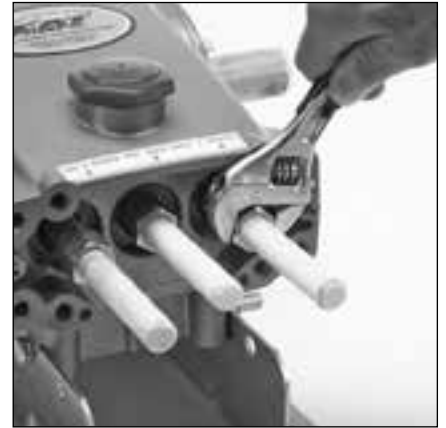
4.2 Use a 7/8" wrench to remove plunger assembly from each plunger rod.
