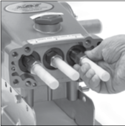
4.4 Install plunger assembly onto each plunger rod.
