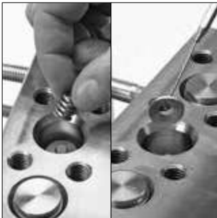
1.8 Place washer over tip of spring retainer and then coil spring.
