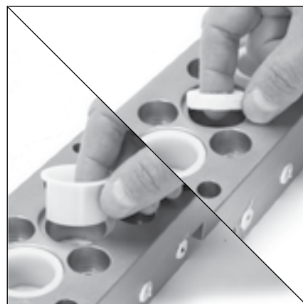
3.12 Remove collars and wicks from crankcase side of housing block.
