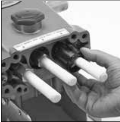
4.1 Remove seal retainers from crankcase.
