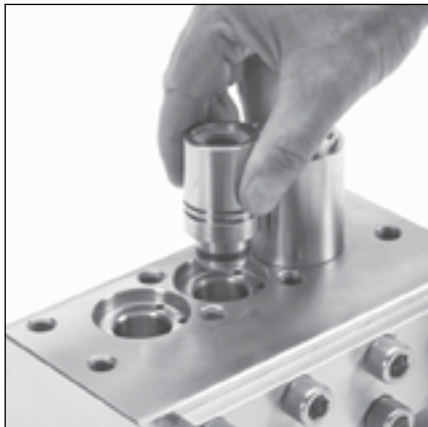
3.8 Remove V/P cylinders from IMDM.
