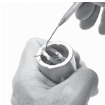
3.11 Remove male adapter from each V/P cylinder.
