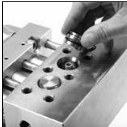
1.9 Press in valve plug into each valve chamber.
