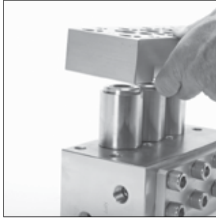
3.22 Position housing block with counter-bore surfaces facing downward over outer cylinders.
