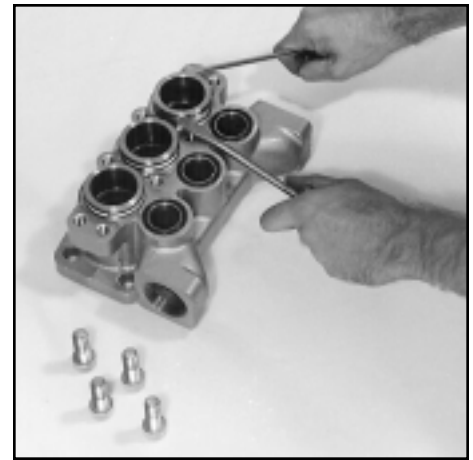
3520, 3521, 3527 Removal of V-Packing Cylinder
