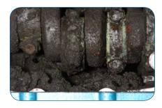
Oil viscosity change shown causing loss of oil lubricity leading to component discoloration and failure
