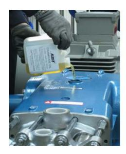
Good lubrication is the simplest, most efficient and least expensive preventative maintenance for your pump. Use only genuine/approved Cat Pumps crankcase oil to extend the life of your high pressure reciprocating pump.
